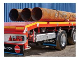
Aluminium ramp basket under the rear cut-out of the loading floor allows for fast and safe transport of additional equipment and increases the loading capacity of the swan neck.
