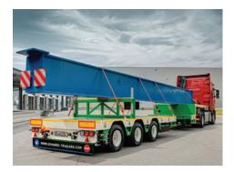
Load trestles are used to level the loading floor with a swan neck. Their number depends on the weight and length of transported elements. It is possible to adjust the shape individually.
