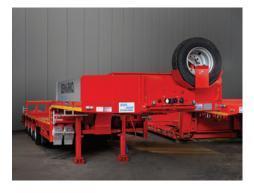
A clamp securing the spare wheel at the front of the semitrailer may hold 2 spare wheels.
