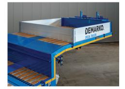
Aluminium side walls, fixed at the front, integrated with a closed tool storage, allow transporting small cargoes or storage of equipment used for loading.
